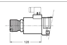
When the set screw is screwed and its point is aligned with the edge of the knob, tighten the knob till it touches the spool: in this position the override is not engaged and the valve is de-energized. After adjusting the override, tighten the set screw in order to avoid the knob loosing.
